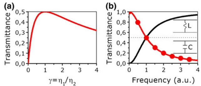
**Fig. 3** **a** The dependence of transmittance on  $\gamma = \eta_1/\eta_2 = n_2/n_1$  shows that the maximal transmittance  $T = 0.5$  is reached when  $\gamma = 1$ . **b** Positive and negative  $\xi$  of a metamaterial is analogous to the high- and low-frequency filters, respectively. Being selected in an appropriate way, they can have equal transmittances and a phase difference  $90^\circ$  at the working frequency
