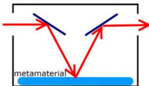
**Fig. 11** The reflection polarizer can easily be converted into the transmission polarizer with the help of additional mirrors. For that the metamaterial layer should preserve its functionality for the incidence at small angles
