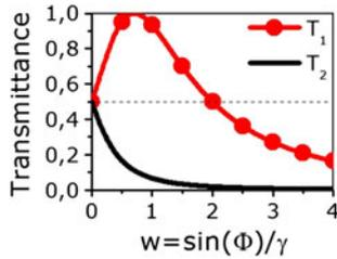
**Fig. 6** There are two solutions for the metamaterial reactances. The first solution (27) can give the transmittance up to 100 %, while the transmittance for the second solution (28) cannot exceed 50 %
