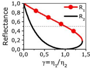
**Fig. 4** There are two solutions for  $\gamma = \eta_1/\eta_2 = n_2/n_1 < \sqrt{2}$ . Both of them have reflectances less than 0.5 for  $\gamma > 1$  and can have large reflectance  $R \approx 1$  for  $\gamma \ll 1$ . Physically this means an incidence from the material with a refractive index  $n_1 \gg n_2$
