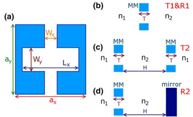
**Fig. 9** a Metamaterial’s unit cell design for polarization converter: view from top. Side view of the polarizer in the transmission (T1) and reflection (R1) single layer (b), transmission double layers (T2) (c) and reflection single layer with ground plane (R2) (d) configurations
