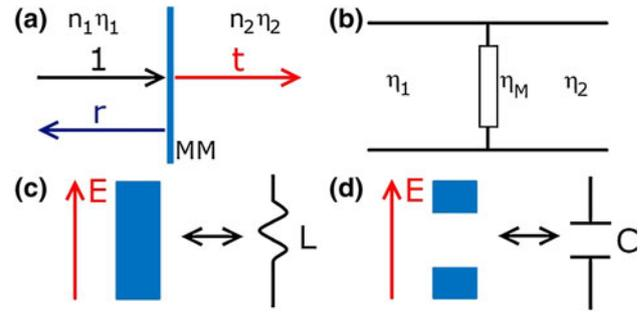
**Fig. 2** Reflection and transmission of a plane wave incident on the metamaterial interface between two dielectrics (a) is equivalent to reflection and transmission of the wave in the connected transmission lines with different impedances  $\eta_1$  and  $\eta_2$  and shunted with a load  $\eta_M$  (b). In the lossless metamaterial a metallic wire along the electric field is an analogue of an inductor (c), while a dielectric gap between two metal parts is equivalent to a capacitor (d)
