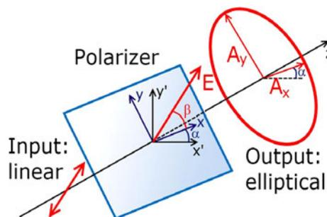
**Fig. 1** Operation principle of the polarization converter. An incoming linearly polarized wave is converted into an elliptically polarized. Rotating the linear incoming polarization with respect to polarizer (angle  $\beta$ ) we can obtain any polarization from linear to circular. Rotating the device together with the input polarization (angle  $\alpha$ ) we can change the orientation of the output ellipse
