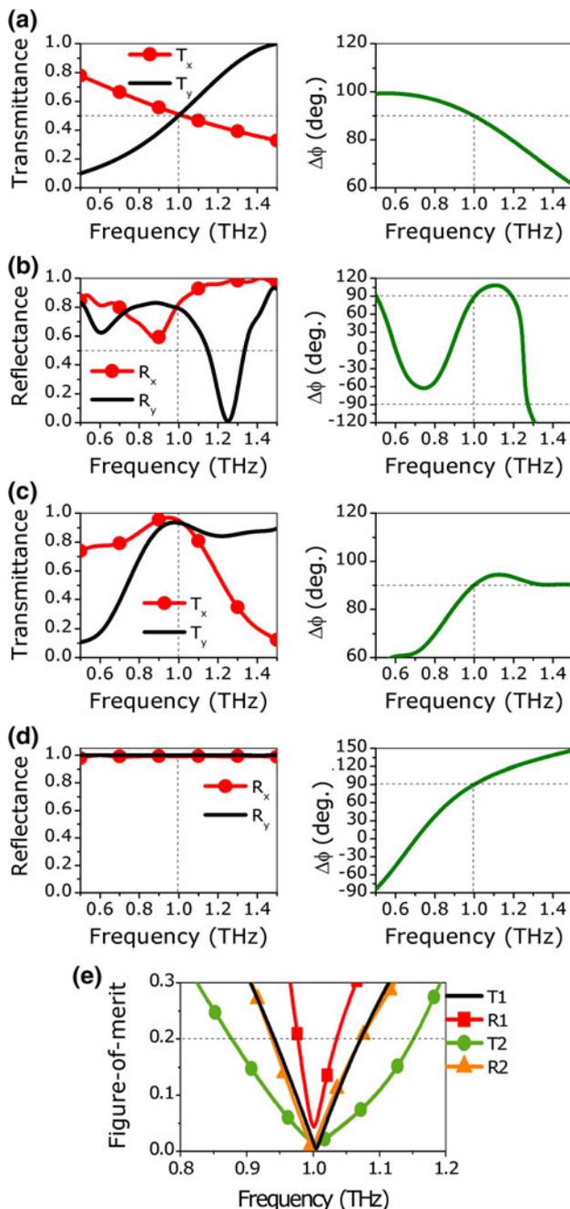
**Fig. 10** Transmittance/reflectance and phase difference for designs **a** *T1*, **b** *R1*, **c** *T2*, **d** *R2* are close to the theoretical maxima. **e** Figure of merit  $\text{FoM} < 0.2$  shows the converter's bandwidth, which is the largest for the transmission through two metamaterial layers (*T2*) design
