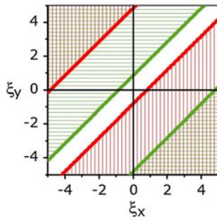
**Fig. 8** The graphical representation of the allowed pairs of metamaterial reactances  $\xi_x, \xi_y$  that give a solution to the dielectric thickness  $H$ . The first and second solution are marked with vertical red and horizontal green lines, respectively. There exist areas where two, one and no solutions are possible. Solutions can be of the same sign
