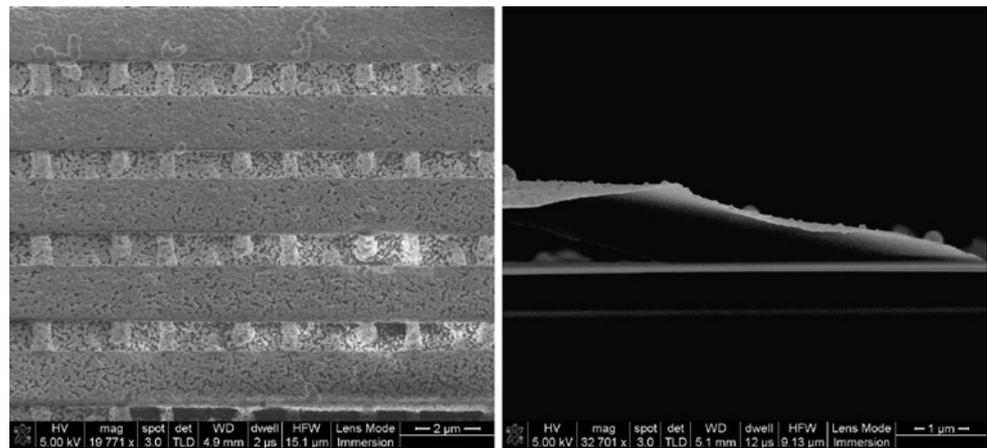
position are presented in Fig. 2a. The Ag layer is deposited not only on the top of the structure but also on its sidewalls. There is still particle formation in the solution followed by their adhesion to the deposited layer, but their influence on the transmission characteristics is minimal and can be neglected. A zoom-in of the 3D covered structure (Fig. 2b) shows the presence of silver layer inside the bulk structure as well.
