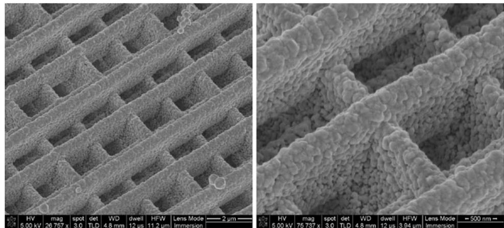
**Fig. 3** (a) Sidewall SEM image of the woodpile. As can be seen, the deposition takes place all through the depth of the woodpile crystal. Here 5 periods in the vertical direction are presented. (b) An example of weak adhesion of the silver layer to the untreated silica surface. It illustrates the importance of pretreatment for a good adhesion
