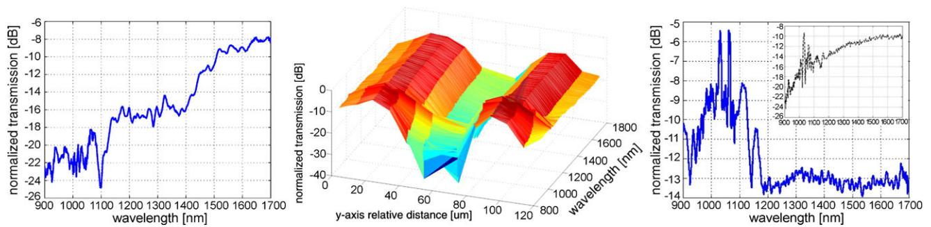
**Fig. 4** (a) The obtained transmission spectra of a polymer woodpile. The two dips at 1100 and 1400 nm are identified as Bragg reflection peaks of the woodpile structure. (b) The spectra obtained while scanning the metallized sample along the  $y$ -axis. The two symmetrical transmission peaks are clearly visible at structure's edges ( $y = 20$  nm
