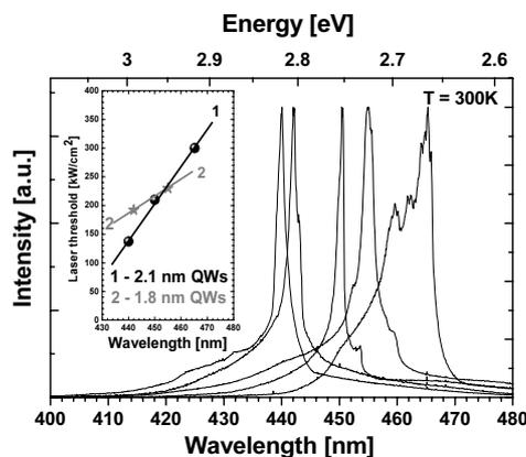
**Figure 3** Emission spectra of different samples above threshold. Inset: laser threshold in dependence on the radiation wavelength for 2.1 nm QWs (1) and 1.8 nm QWs (2).
