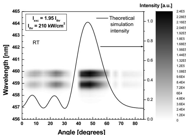
**Figure 2** Density plot of spectral-angular distribution of the laser emission in the far-field and calculated intensity distribution for the 5<sup>th</sup> order transversal mode.
