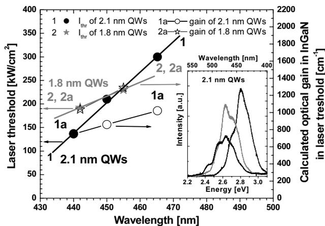
**Figure 4** Laser threshold (1, 2) and calculated optical gain of InGaN (1a, 2a) dependences on wavelength for 2.1 nm (1, 1a) and 1.8 nm (2, 2a) QWs. Inset: PL spectra of 2.1 nm QWs at high excitation level.
