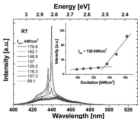
**Figure 1** Emission spectra of the sample with 2.1 nm QWs in dependence on excitation intensity. Inset: emission intensity versus excitation intensity.
